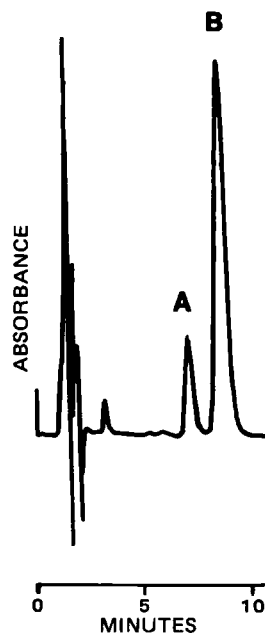
Figure 1 —Chromatogram of a commercial sample of digoxin injectable solution showing the contaminant, 2-mercaptobenzothiazole (A), and digoxin (B). The mobile phase was 29% acetonitrile; the detector was set at 218 nm.
